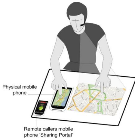
Figure 3. Two handed interaction with the projection and the physical mobile phone. Here the projector is in the form factor of an ear worn device which communicates with the mobile phone wirelessly. The mobile phone is placed within the projection space, and can be used as normal.
