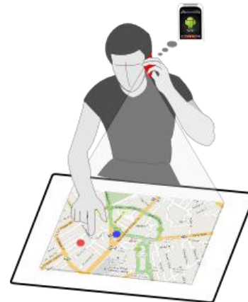
Figure 1. Touch interaction during a phone call. A projector in the bottom of the phone combined with camera allows the projection of and interaction with the mobiles interface. Here Jack provides his friend Tony with turn by turn directions to his house. The red dot indicates Tony's current location, the blue dot indicates the destination.
