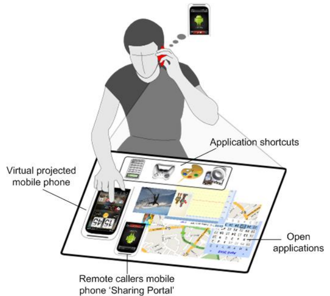
Figure 2. Interaction during an active phone call. The user can interact with the phone by touching the virtual interface. Shortcuts provide access to frequently used applications. The large display presents multiple applications, alternative visualization of information and desktop interaction paradigms.
